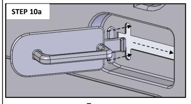
**STEP 10a:** Install the Door Handle [INS-TERRAIN-HANDLE] into the Door/Frame Assembly [04627V-A] from the exterior of the panel. Insert the tabs near the latch on the Door Handle into the slot as shown. Slide the partially installed handle towards the door frame.
