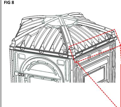
**STEP 8:** Finish fastening the Range Roof assembly to the assembly with (10) Bolt  $\frac{1}{2}$ 0 x 1- $\frac{1}{2}$ 1 [2020], (10) Washer  $\frac{1}{2}$ 1 ID  $\frac{1}{2}$ 6 OD [3014], and (10) Wing Nut  $\frac{1}{2}$ -20 [6013]. Fasten through the two outer holes on each roof panel and the slots on the wall/door panels.
