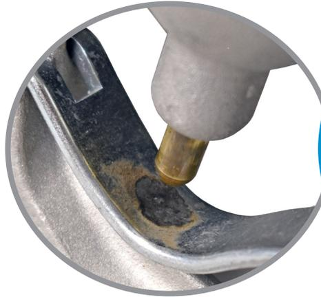
Metal on metal contact creates friction and quickly wears surfaces.
