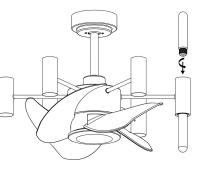
Holding gently the lamp arm, take a glass shade and install it over the bulb turning it clockwise. Tighten. Install the other 11 glass shades.
