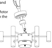
5. Insert the Down Rod into the Yoke making sure that the wires are not twisted and aligning the holes for the pin on the Down Rod with the holes in the motor Yoke. Insert Pin all the way
