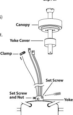
4. Thread the wires and safety cable that comes from the Motor assembly through the Down Rod.
