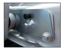
Tighten the button head with an M5 allen wrench and the other bolt with a 10mm wrench.
