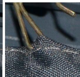
Impale the fabric and hang the hook on the sliding block S6
