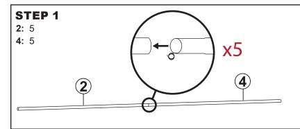
**TIP:** To avoid pinching your fingers, angle the tube with the torsion spring so the spring is on the inside the other tube, then align the tubes so they are straight and push them together.
