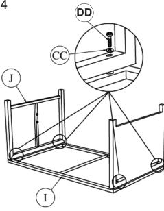
Do not fully tighten hardware until after Step 9 is complete.
