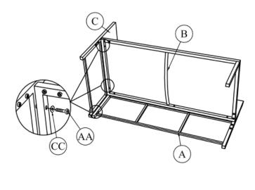
Do not fully tighten hardware until after Step 7 is complete.
