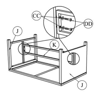
Do not fully tighten hardware until all components in this step have been connected.
