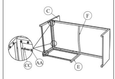
Do not fully tighten hardware until after Step 7 is complete.
