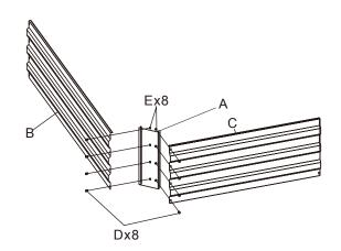
② Do the same way to other 3 frames and panels. Tighten bolts and nuts with Allen Key (F).
