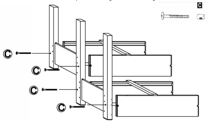
Step 5 Slide in bottom panels 10, 11, 11, and 10 through both side of the frame's panels 8 and 9.
