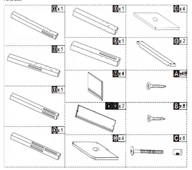
Note: There are two panels of part 8 and two panels of part 9.
