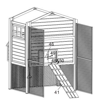
• Following below diagram, fix 2pcs Post 5 (#5), 2pcs Pen Mesh Panel (#23) and Post 6 (#6), Post 7 (#7) in turn. Requires totally 24pcs M6x30 Bolt (#48) and 24pcs M6 Nut (#50)
