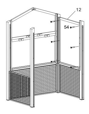
Same as Step 4, assemble Coop Left Panel (#13) between Posts #2 and #4 by 6pcs Self-tapping Screw 4x30 (#54).
