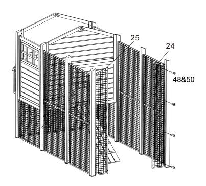
• Assemble the Pen Door Panel (#26) between above two side panels, by 4pcs M6x30 Bolt (#48) and 4pcs M6 Nut (#50) on each side.
