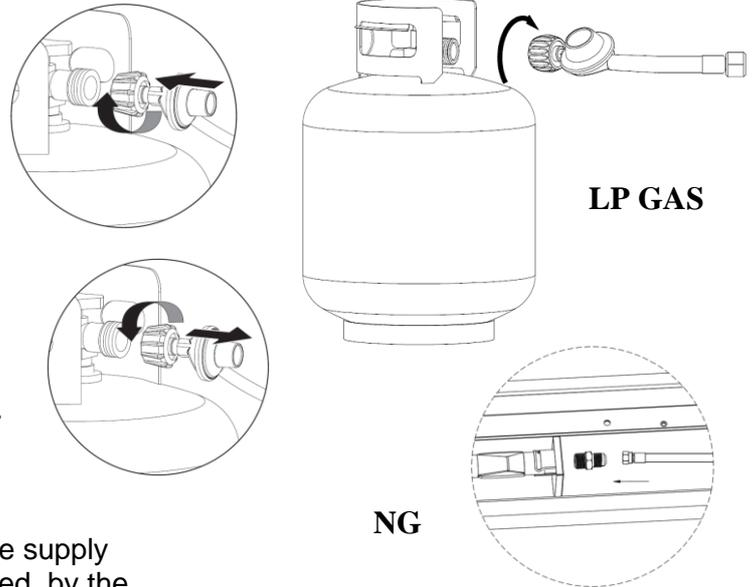
The appliance must be isolated from the gas supply piping system by closing its individual manual shutoff valve during any pressure testing of the gas supply piping system at test pressures equal to or less than 1/2psi (3.5kPa)
