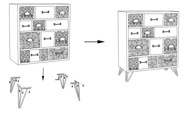
Tighten each screw firmly. DO NOT over tighten any of the screws as this may cause stripping. When using power tools, be careful not to damage the wood.
