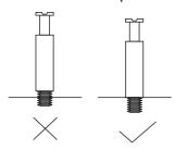
Below shows how the pins are used to assemble the panels together.
