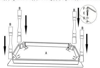
**Step 2** Conbine wooden bottom© and legs(B), then tighten them by long screw(E) and round washer(D).
