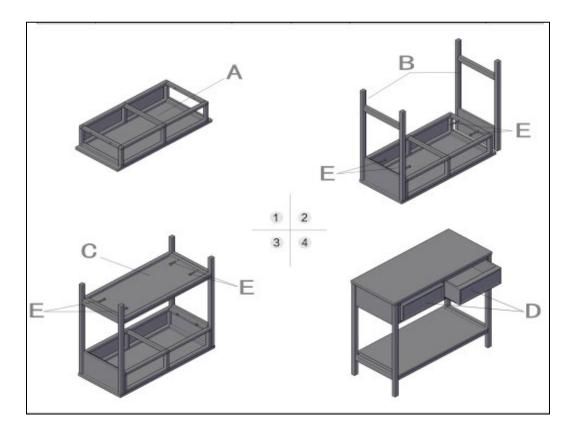
Tighten each screw firmly. DO NOT over tighten any of the screws as this may cause stripping. When using power tools, be careful not to damage the wood.
