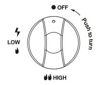
5. When burner is lit, turn the control knob to desired heat output position between "LOW" and "HIGH".
