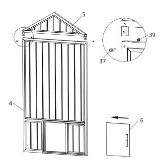
• Assemble the (#4) & (#5) combination part into the Coop by Bolt (#37), and Nuts(#39), next to (#3).
