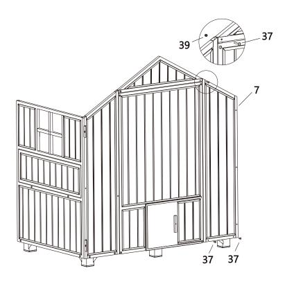
• Attach the Coop Right Wood Panel (#8) by Bolt (#37). Then fix the rest 2pcs of Coop Connecting Metal (#32) with Bolt (#37) on the right edge of the front panel.
