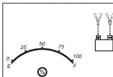
If the clamps are INCORRECTLY connected with regard to polarity, the LCD screen will display the following (the "+" and "-" inside the battery icon will flash and the clamp icons, the battery icon and the gauge without the pointer will light) and a warning will sound until the clamps are disconnected:
