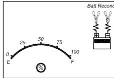
The battery recondition indicator, the clamp icons, the battery icon and the gauge without the pointer will light solid, the bars on the battery icon will change from solid to empty (top to bottom) repeatedly and the battery recondition icons will flash.
