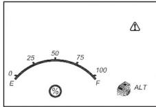
The fault icon and "ALT" will flash; the alternator icon, and the gauge without the pointer will light solid.
