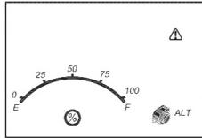
The fault icon and "ALT" will flash; and the alternator icon, and the gauge without the pointer will light solid.
