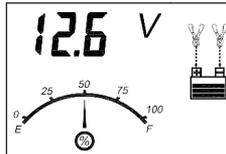
The digital display shows the current voltage of the connected battery for 10 seconds. During this period, pressing the battery voltage check button again will return the unit to charging mode.
