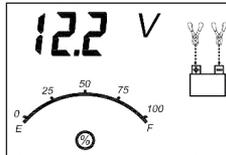
The digital display shows the current voltage of the connected battery for 10 seconds. During this period, pressing the battery voltage check button again will return the unit to standby mode. The gauge without the pointer will light solid. The unit will automatically return to standby mode after 10 seconds.
