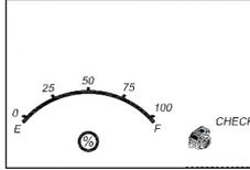
"Check" will flash, and the alternator icon and the gauge without the pointer will light solid.
