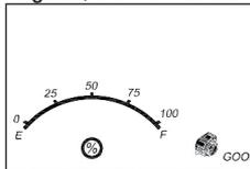
"Good", the alternator icon and the gauge without the pointer will light solid.
