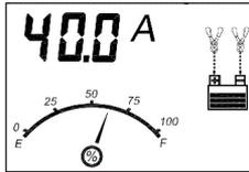
The digital display shows the output current that is charging the battery. The gauge indicates the charge status of the battery. The clamp icons and the battery icon light solid, the bars on the battery icon will change from empty to solid (bottom to top) repeatedly and the arrow icons will gradually and repeatedly move downward to the battery icon.
