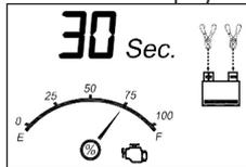
The digital display shows the countdown.\* The battery charge gauge will indicate the battery's current charge status. The engine start icon flashes. The clamp icons and battery icon light solid, and the bars on the battery icon will change from empty to solid (bottom to top) repeatedly and the arrow icons will gradually and repeatedly move downward to the battery icon.
