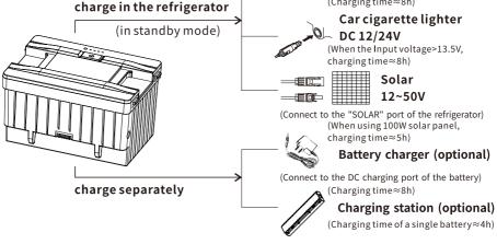
**Note:** It is suggested to switch off the refrigerator when charging the battery (the power supply may mainly power the compressor when the refrigerator is running).
