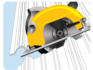
Sawing the panels Figure 4
