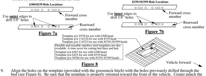
bed (see Figure 8). Be sure that the template is properly oriented toward the front of the vehicle. Center punch the holes that will be used to cut the opening in the bed. If the vehicle is equipped with a bed liner, a section of the bed liner must be cut away so that the gooseneck hitch can contact the bed corrugations.
