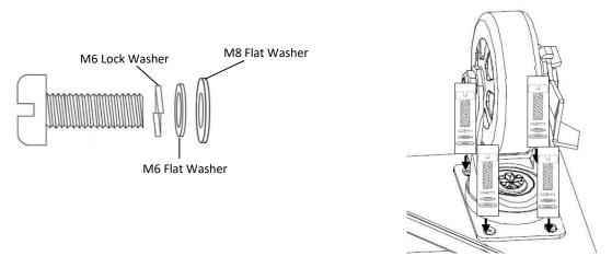
(2) Total 16 pieces M6\*15 Screws (Note: Lock Washer and Flat washer are not needed)
