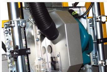
Makita Saw on a Spinning Insert Plate w/Dust Collection
