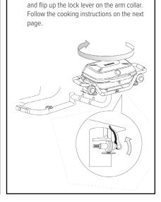
Rotate the grill head to the desired position
