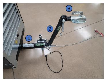
Ensure the hitch attachment, section three, is parallel with the trailer lead, section one, when installed. This will ensure the unit stays mounted on the hitch and undue stress is not placed on the trailer.
