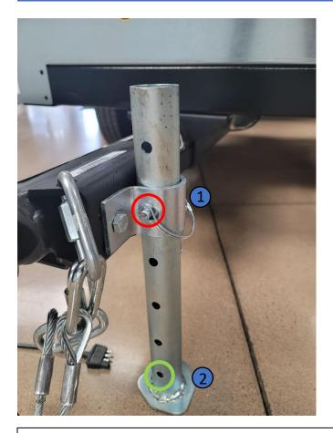
After the trailer support leg is locked into place, **YOU MUST** install the safety cables as shown. Safety cables should be installed straight and should not cross.
