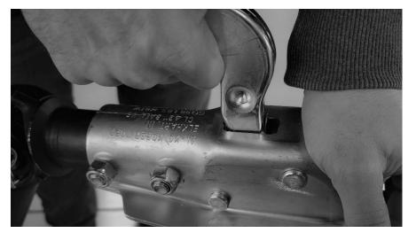
To detach trailer from towing vehicle, ensure trailer wheels are properly chocked (REF pg. 26), and on a flat and level surface. Lower the trailer support arm and lock it into place utilizing the supplied pin. Disconnect the trailer power supply and trailer safety cables. Firmly grasp the trailer release handle and pull up ward. This will disconnect the trailer ball mount from the towing vehicle ball hitch.
