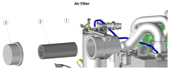
Since the air cleaner/filter used on this engine is a dry type, DO NOT apply oil to it.
