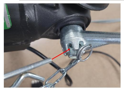
Once the trailer arm is in the correct position, tighten the adjustment handles and replace the cotter pins. Ensure to firmly press the cotter pins in place, and verify they go into one of the holes in adjustment bolt, such as the one shown on the left.
