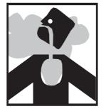
DANGER: Death or serious injury can result from asphyxiation. Running engines produce carbon monoxide (CO), a colorless, odorless poisonous gas. CO generated by the engine can rapidly accumulate even in areas that appear to be well ventilated. This CO accumulation can result in dangerous and FATAL concentrations within minutes.
