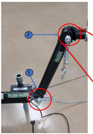
Height and angle can be adjusted at these two locations. They work by having locking teeth that press together at various positions to give you a perfect fit for your application. Begin by removing the cotter pin at each location. Once the pin is removed you may loosen and adjust by turning the handle counterclockwise far enough to allow the teeth to disengage and move without grinding against each other.
