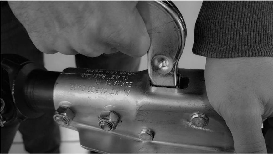
To detach trailer from towing vehicle, ensure trailer wheels are properly chocked (REF pg. 26), and on a flat and level surface. Lower the trailer support arm and lock it into place utilizing the supplied pin. Disconnect the trailer power supply and trailer safety cables. Firmly grasp the trailer release handle and pull upward. This will disconnect the trailer ball mount from the towing vehicle ball hitch.
