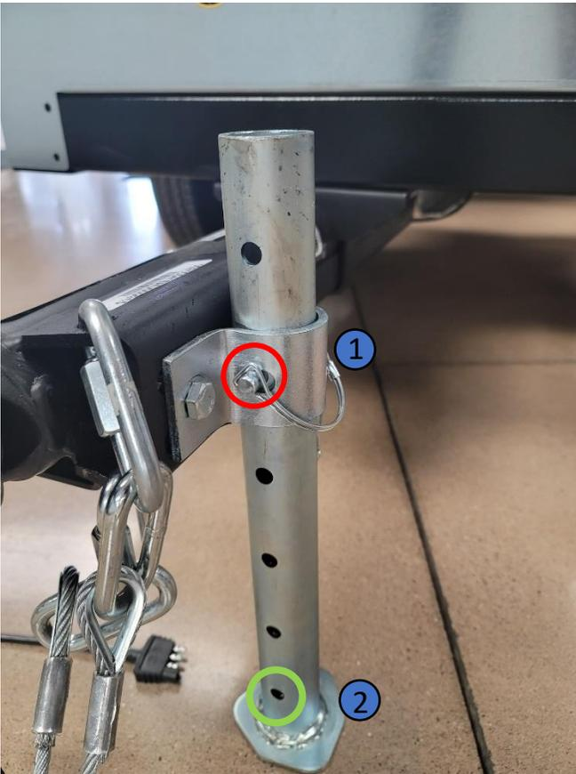
Once the trailer hitch is locked securely in the hitch mount, you will need to raise the trailer support leg to travel height. Begin by pulling the retaining wire off of the pin holding the leg in place (pin and retaining wire marked as 1 in the drawing). Slide out the pin. Pulling upward from the top of the leg, raise the leg to travel height, marked as figure 2. Replace the pin ensuring to use the retaining wire to lock the pin in place.
