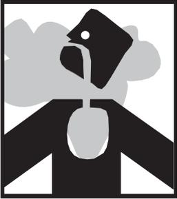
**DANGER: Death or serious injury can result from inhaling compressed air without using proper safety equipment. See OSHA standards on safety.**
