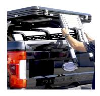
Open the lock mechanism and lift up the tent. The tent will automatically open.
