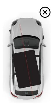
Make sure the tent is centered with the vehicle to keep it balanced at all times. This will help maintain the vehicle safe at higher speeds.
