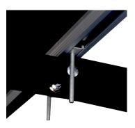
Place a plate under the crossbar aligning the holes with the bolts.
