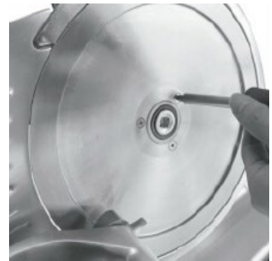
3. Loosen the screws of the blade
