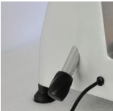
1. Loosen the blade cover locking knob to release the blade
