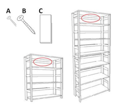
**STEP 2a**: Attach the Strap(**C**) to the highest cross brace that spans the back of your bookcase with 2 Small Screws(**A**).
