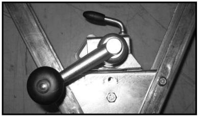
Secure item 2 (tongue jack mounting bracket) with item 3 (5/16 Allen HD Cap Screw) to the tongue connection bracket or mounting bracket
