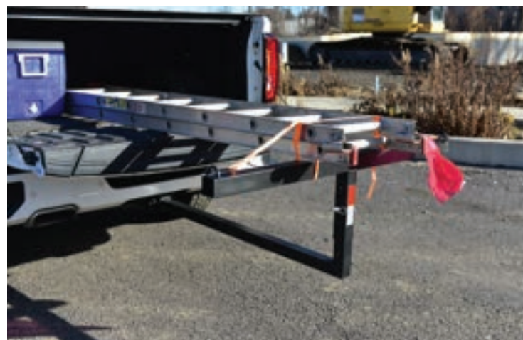
Horizontal tailgate support adjusts from 17" to 23-3/4" above the hitch
