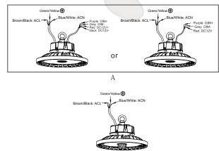
Installation Methods: Hook Mount, Ceiling Mount, 1/2"NPT Mount.(Please choose the most suitable installation method for the purchased produdct as per your needs)
