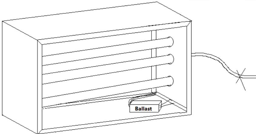
Disconnect power to luminaire or circuit (if possible). Ensure all power is off by using a voltmeter or other method to confirm.
