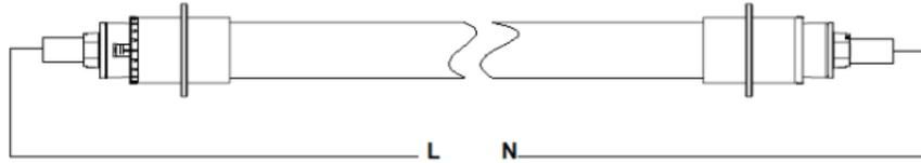
b. Power cord installation, please rewiring the fixture according to the below diagram.
