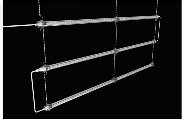
Our new and revolutionary SignStorm Sign tube Offering significant energy-efficiency and lifetime improvements over fluorescent lamps. SignStorm lamps are installed by bypassing existing fluorescent ballasts, and hard-wiring tombstone lamp-holders directly to incoming AC power leads. Dual-ended bypass lamps eliminate the need to replace shunted tombstone lamp-holders in existing fluorescent luminaires. AC power code is also provided for new installation.
