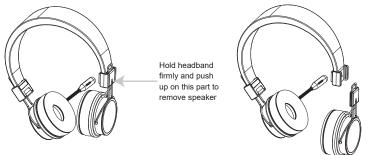
When you re-attach the right speaker, the Elite Plus™ becomes a binaural (dual speaker) headset with high fidelity stereo sound when playing music. To ensure a positive connection, make sure the speaker connector (plastic part with "UP" arrow) is fully seated on the headband with a positive 'click'.
