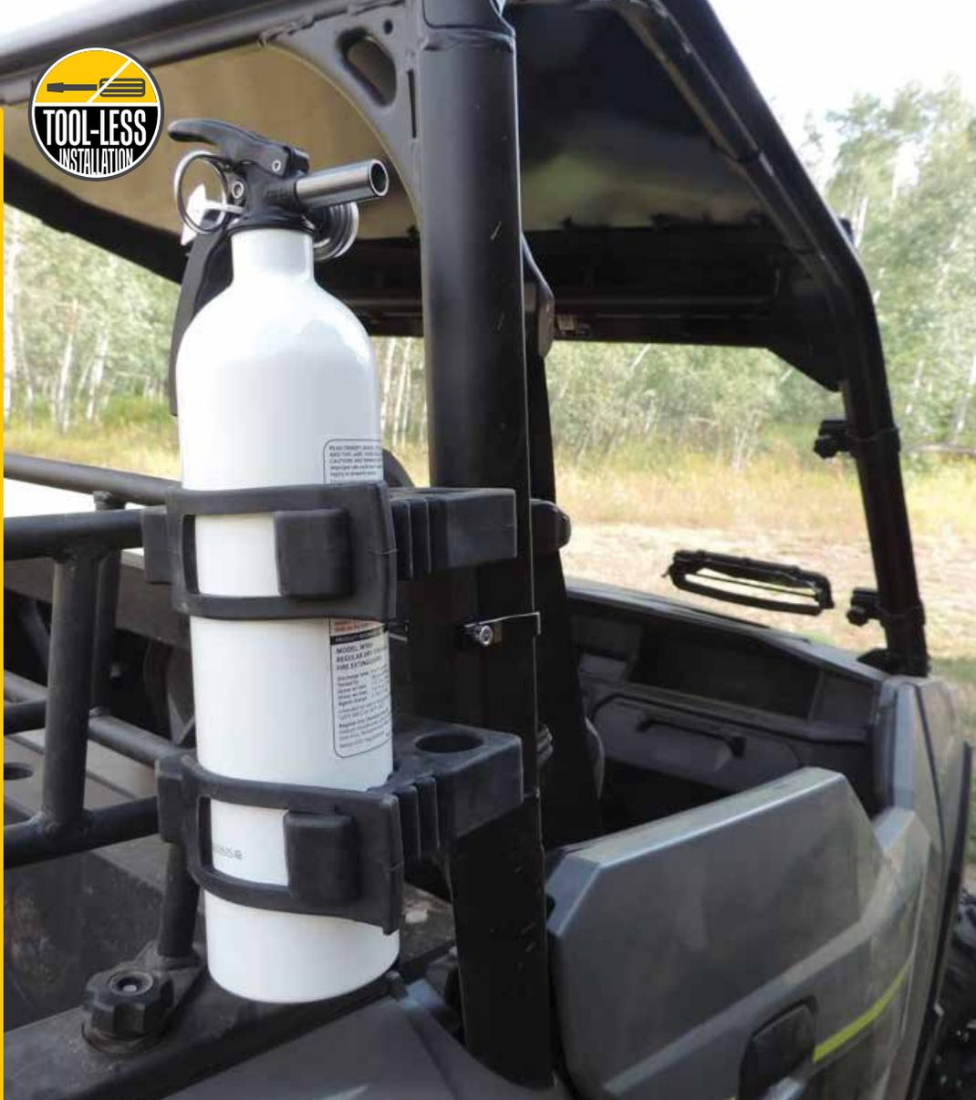
The Hornet Fire Extinguisher UTV Roll Bar mount comes equipped with two heavy rubber grips attached to two large roll bar clamps, making it a simple task to install a fire extinguisher on your UTV.
