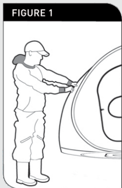
STEP 1: Remove all stakes and tie downs. Close all windows and doors. Lay blind flat on its side.
