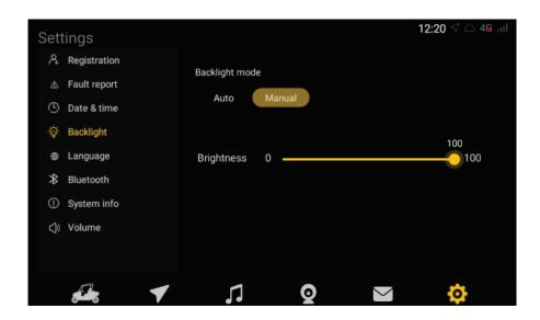
Automatic brightness is adjusted based on the current headlight state. If the headlights are on, it is considered to be night and the screen brightness is dimmed. If the headlights are off, it will be considered daytime and the screen brightness will be increased automatically.
