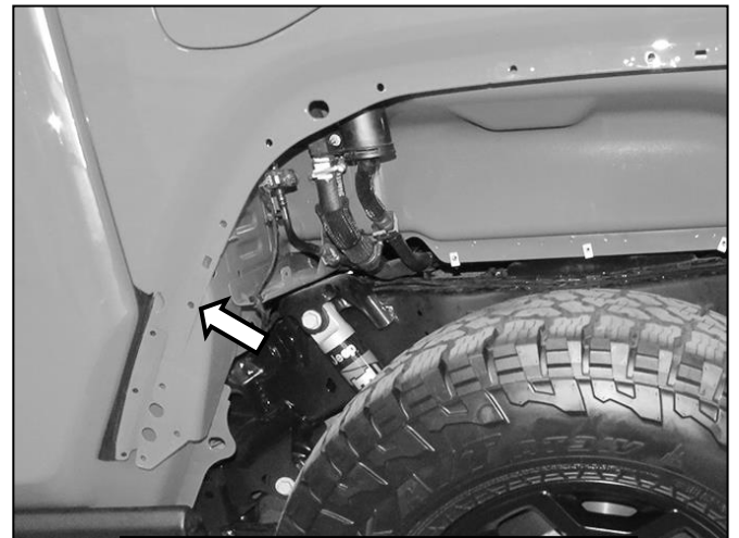
(Fig 4) Drill the hole in the front of the wheel well with a 25/64" drill bit
