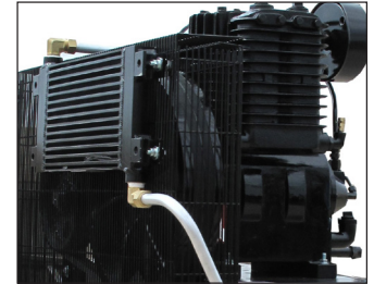
Air cooled after cooler Elite unit
