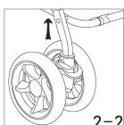
5. Assemble front wheels: Insert each wheel onto the respective leg and push upward until you hear a "click".
