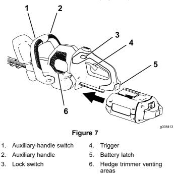
4. Place 1 hand on the trigger handle. Place the other hand on the auxiliary handle (Figure 7).
