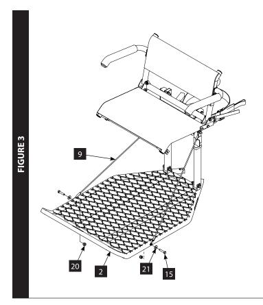
3. Bolt cables (9) onto platform (2) using two provided 5/16-18 x 1-1/2 bolts (15), two steel washers (21) and two 5/16-18 locknuts (20). **SEE FIGURE 3. You must now tighten all nut & bolt assemblies. Be sure not to over tighten or crush tubing when tightening!**
