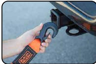
2. Attach the other end of the strap to the vehicle you are using to tow with. Many vehicles have hooks or loops you can use, but if you do not have one, find a part of the frame of the vehicle. The cross member beneath the engine may be the best area to attach a tow strap.
