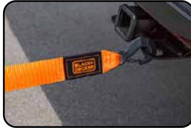
3. Once the strap is attached to both vehicles, pull the tow vehicle away slowly to take out the extra slack in the strap. Once the strap is taut, slowly accelerate at very low speed until the disabled vehicle starts moving.
