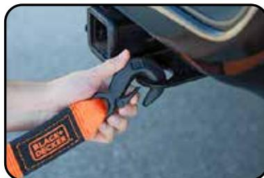
1. Connect the strap to the machine / vehicle that is disabled. Make sure to secure to a vehicle's tow hook, or a part of the frame so that it does not damage the vehicle.
