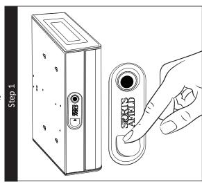
2. Insert the backup key. Turn the key clockwise and your vault door will unlock.
