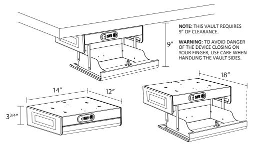
In order to mount the vault flush to the edge of your desk or desired surface, use the provided template and complete the following steps for mounting. Keep in mind, when the vault drawer is fully open it will extend 6" beyond the edge of your desk so that you may easily and quickly access the contents.
