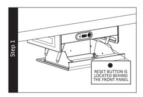
Press the reset button to start the programming process. You will hear one beep and the indicator ring will illuminate on the front of the door.
