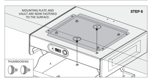
• Locate the (2) thumb screw holes on the top, inside of the vault. Hold the unit in position and use (2) thumbscrews to fasten the unit to the mounting plate.
