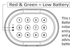
This safe is equipped to alert you of Low Battery Mode. This Low Battery Warning is initiated immediately after a successful code entry. The keypad will illuminate both the red and green LED lights for 3 seconds. It is highly advised to immediately replace the safe's batteries to avoid being locked out of your safe.
