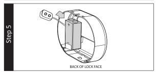
**WARNING:** The batteries must be inserted with the correct polarity. Exhausted batteries must be removed from the product and discarded safely. Do not mix old and new batteries. Do not mix alkaline or standard (carbon – zinc) batteries. Do not use rechargeable (nickel – cadmium) batteries.
