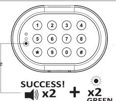
Inactivity Timeout: If this programming sequence is not completed within 10 seconds the red LED will flash 3 times and the keypad will shut down.
