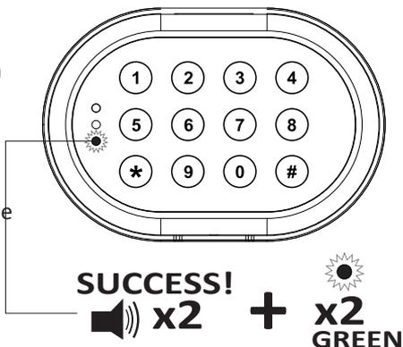
**Inactivity Timeout:** If this programming sequence is not completed within 10 seconds the red LED will flash 3 times and the keypad will shut down. Return to step 1 to restart this process.
