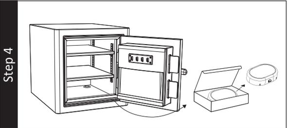
5. Locate the 1x9V battery. Install into the battery compartment on the back of the lock face in the proper orientation. The keypad will beep when batteries are successfully installed.
