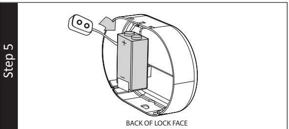
**WARNING:** The batteries must be inserted with the correct polarity. Exhausted batteries must be removed from the product and discarded safely. Do not mix old and new batteries. Do not mix alkaline or standard (carbon – zinc) batteries. Do not use rechargeable (nickel – cadmium) batteries.
