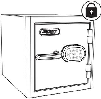
1. Three consecutive rejected security code entries puts the safe in "Basic Lockout" mode. The keypad is deactivated for 30 seconds.
