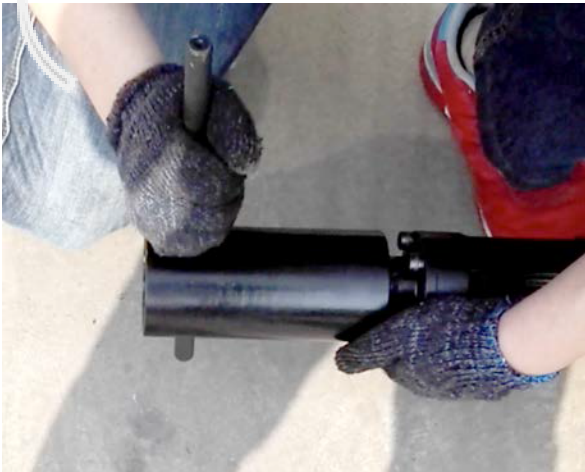
Fig. 3 ) Insert Socket Pin, then rotate Piling Socket Sleeve \Phi 69 to make sure it is tight & secure.!
