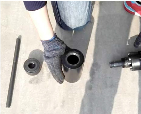
Fig. 1 ) Identify Post Driver, Piling Socket Sleeves (2 pieces), Inner Post Head and Socket Pin.!
