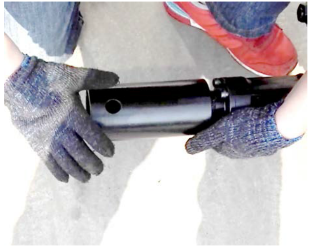
Fig. 2 ) Attach Piling Socket Sleeve by screwing it onto Post Driver.
