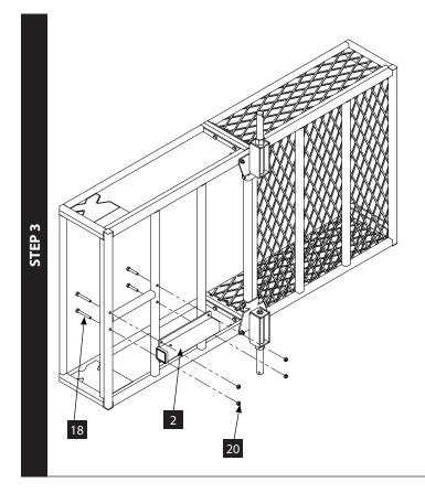
3. Attach the tongue receiver (2) to the front trailer frame (5) using two 5/16-18 x 2  $\frac{1}{2}$  IN bolts (18), two 5/16-18 x 1  $\frac{3}{4}$  IN bolts (17), and four nuts (20).
