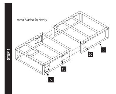
1. Attach front and rear trailer frames (5 & 6) using four 5/16-18 x 2  $\frac{1}{2}$  IN bolts (18) and nuts (20).
