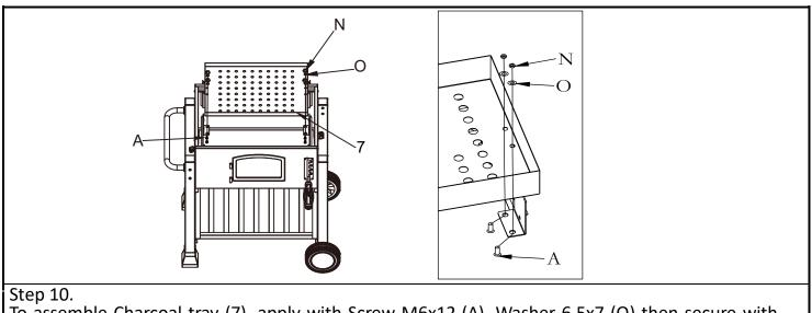
To assemble Charcoal tray (7), apply with Screw M6x12 (A), Washer 6.5x7 (O) then secure with Nut M6 (N).
