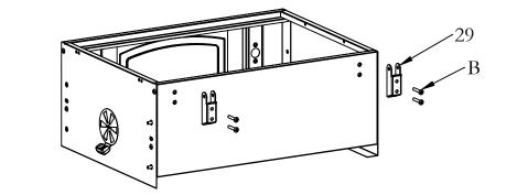
Step3. Assemble the Lower hinge (29) with Screw M6x35 (B).
