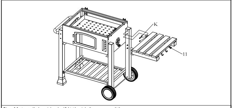
Step11. Install the side shelf (11) with Step screw (K).
