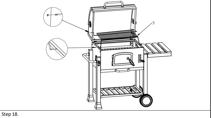
To install the Warming rack (5), plug the four ends of the warming rack into the relative holes on lid and fire bowl respectively.
