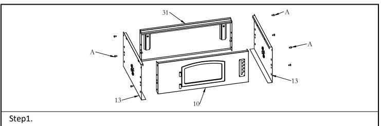
Assemble Fire bowl front panel (10), Fire bowl back panel (31), and 2 pieces of Fire bowl side panels (13) with Screw M6x12 (A).
