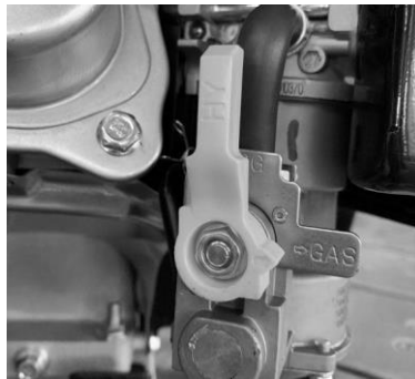
Turn the Fuel Selector to Gas
