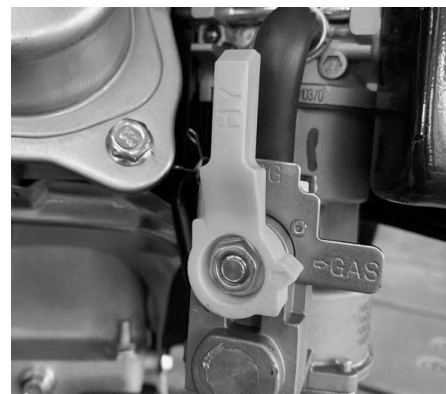
Switch to Gas position
