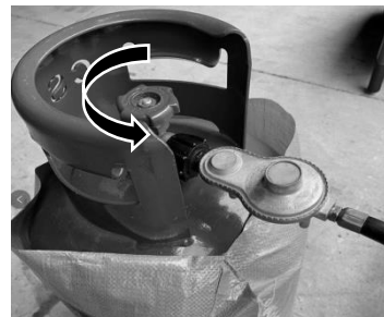
Open the propane tank valve
